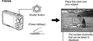
When the focus and exposure are locked, the green lamp lights up, and the shutter speed and aperture value are displayed.
